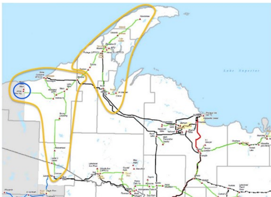
Map shows ATC's transmission system in the western Upper Peninsula. The gold circles indicate how the load pocket will be split into two radially fed areas. Location of White Pine Unit 1 circled in blue on upper left of map. | MISO
